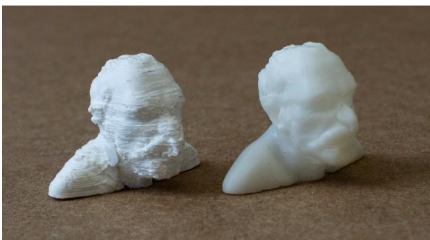
Figure 5: Comparison between PLA printing (left) and resin printing (right)
